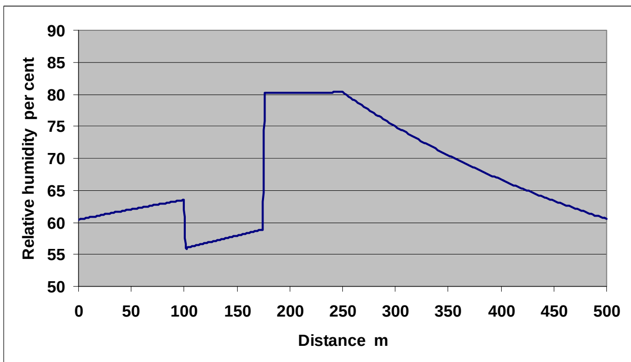
Figure 16.3 Graphical output for relative humidity along the airway.
